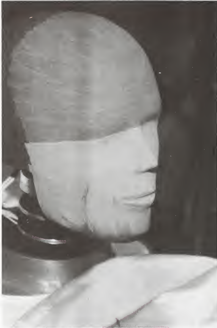
FIGURE 12 -- Right Side Chalk Removal Pattern for System A Positioned 3" Closer
